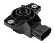
BEI Sensors Model 9970 Hall Effect rotary position sensor is available in two standard output configurations (0-5 V ratiometric or 4-20 mA) for ease of specification and use. Both versions use a standard Amp, Superseal three terminal connector and are available with 12 active angle ranges, 30 degrees up to 360 degrees (in 30 degree increments) in a single output device. Unlike comparable sensors the 9970 can use the full 360 degree travel range making it extremely versatile.
