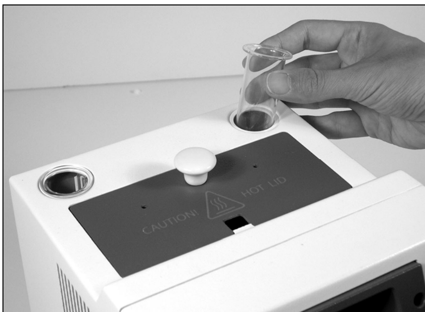
Figure 3. Mounting the glass Capillary Holders.
